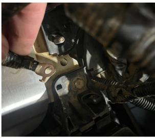
8. Drop in the side bracket aligning with the 6mm nutsert, this should be visible from the inner guard.
