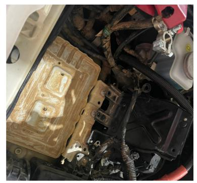
5. Place the Rogue M.O.L.L.E bracket into the cradle, to fit lift the ECU mounting bracket away from the studs and slider the Rogue MOLLE plate in place.
