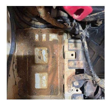
3. Relocate the earth lead to the front ECU bracket, you will need to use this mount when re-assembling the ECU mount.
