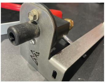
10. Loose fit the isolator side bracket to check from cable clearance the remove to fit battery. Take this opportunity to tighten the front and rear nuts ready for battery to be fitted.
