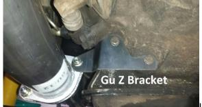
Using the original turbo dump pipe gasket, nuts and bolts install the dump pipe and finger tighten the nuts and bolts. **DO NOT TIGHTEN FIRMER YET.** You will also need to finger tighten the 12mm bolt for the bracket on the dump pipe to the engine block.
