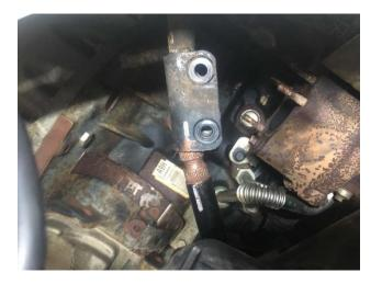
5. IT can be easier to remove the OE cat if the bracket around the cat is removed. Or unbolting the bracket is also possible.
