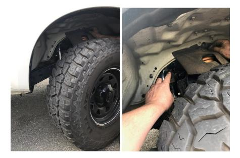
4. You' will need to disconnect the steering column shaft at the knuckle. This will allow you to remove the dump pipe.
