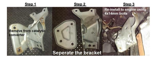
6. Ensure any damaged exhaust mounts are replaced at this time (or you may void your warranty) to prevent future problems (vibrations, rattling or breakage) once the new exhaust is fitted.
