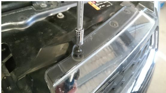
6. Next remove the screws under the wheel well connected the front bar.
