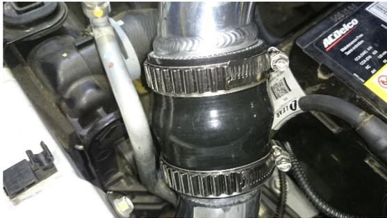
18. Ensure the silicone is pushed all the way onto the ribbed outlet and tighten up all hose clamps firmly.
