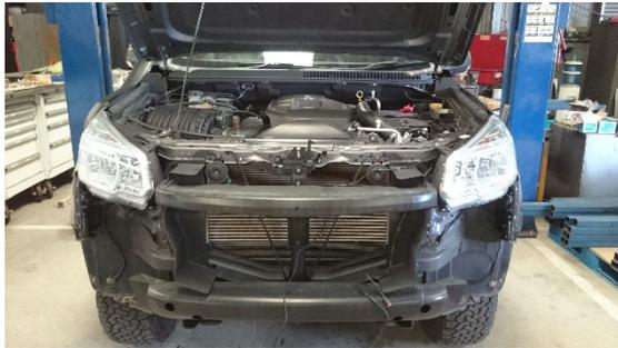
11. Remove the covers over the airbag sensors to gain access to the ducting and reinforcement bar.
