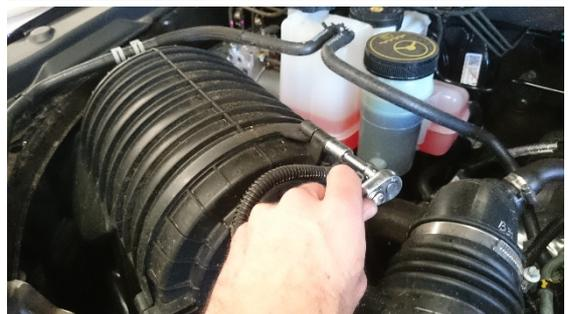
21. Undo the hose clamps from the top of the intercooler.
