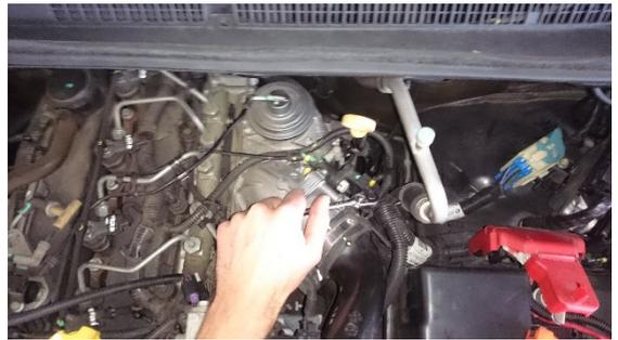
25. Unbolt and remove the OEM intercooler.
