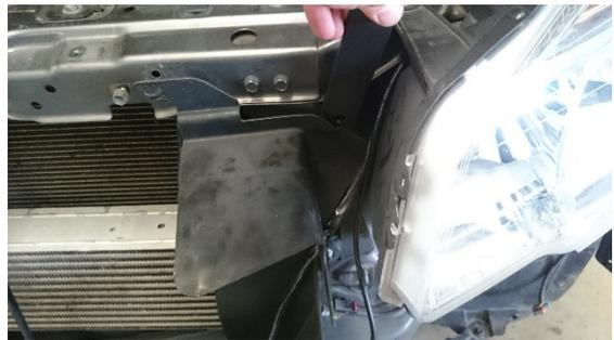
15. Remove the lock panel cover support rods.
