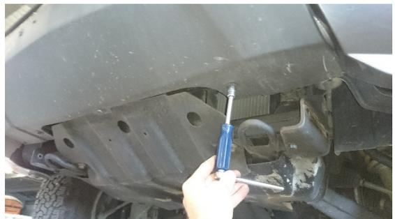
9. After all screws are undone carefully pry the bumper using trim removal tool. It is recommended to have a second person to help hold the bar to prevent damaging the bar during removal.
