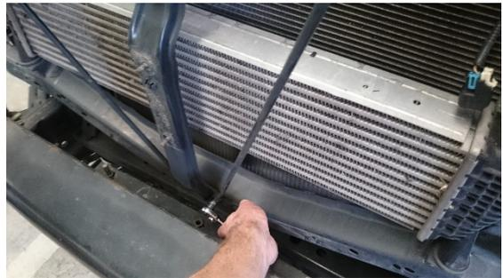
16. Remove the bonnet latch brace and unclip the sensor from the back side of the brace
