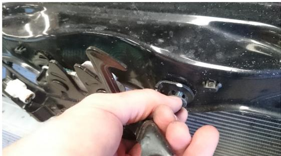
18. Unbolt the lower reinforcement bumper bar in 4 places. (2 on each side)
