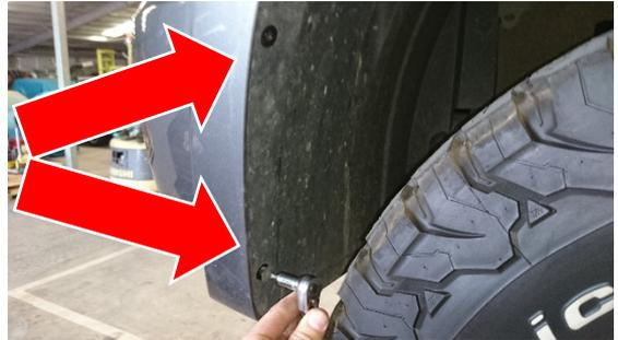
7. Disconnect fog lights if fitted at this stage.
