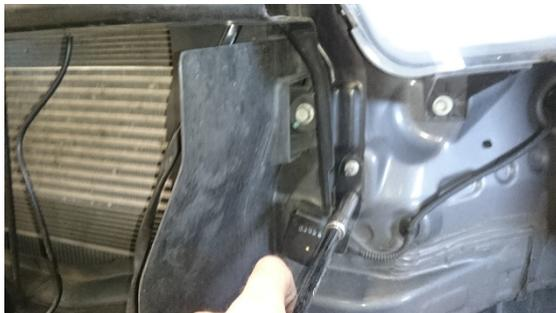
12. Undo the last two bolts in the middle of the reinforcement bar and remove.
