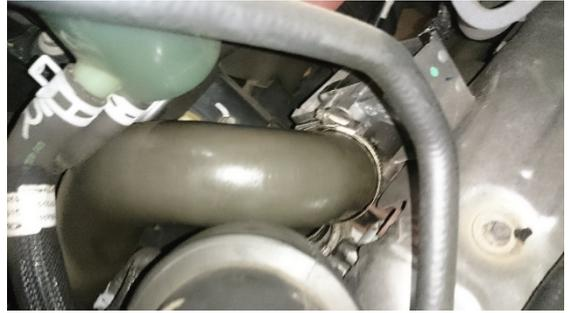
24. Undo and remove the cold pipe from the throttle body.
