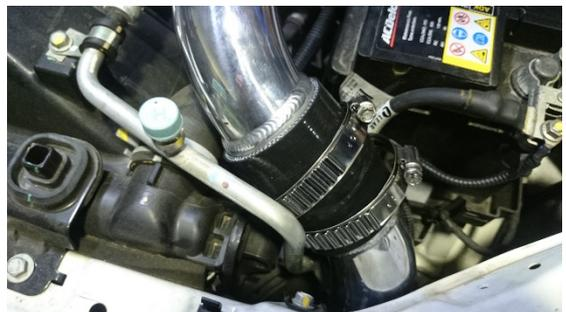
17. Slip the top cold pipe 04.64553 into position and rotate silicon and aluminum piping to make sure that nothing is rubbing.
