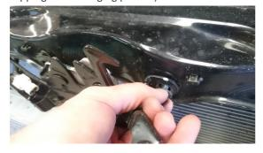
18. Unbolt the lower reinforcment bumper bar in 4 places. (2 on each side)
