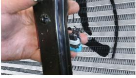
Undo the bolt in the center of the horn and rotate the bracket around so that the plugs do not hit the intercooler when reinstalled.
