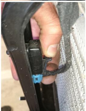
17. Remove bonnet latch and rest to the side (NOTE - it is recommended to temorarily secure with zip tie if required to prevent it slipping and damaging panels.)
