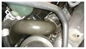
24. Undo and remove the cold pipe from the throttle body.
