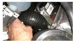
13. Install the hot side LEGENDEX 01.64553 hard pipe into the 135 degree elbow and slip into the 2 inch hump hose on the intercooler at the same time.
