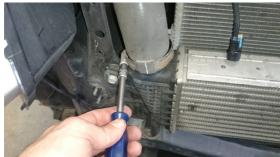
22. Remove the clamps that retain the OEM Rubber intercooler pipes from the steel hard pipe. Then undo and remove the pipes from the radiator core support panel.
