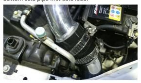
17. Slip the top cold pipe 04.64553 into position and rotate silicon and aluminum piping to make sure that nothing is rubbing.
