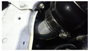
19. It is recommended to use a socket that has a universal joint and appropriate extensions to get to the hard to reach hose clamps behind the radiator core support panel.
