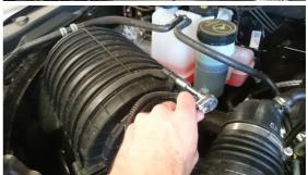
21. Undo the hose clamps from the top of the intercooler.
