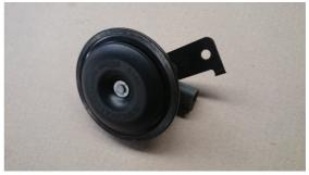
Screw the horn on with the aluminium spacer behind the bracket to clear the lip on the radiator core support panel and connect plugs
