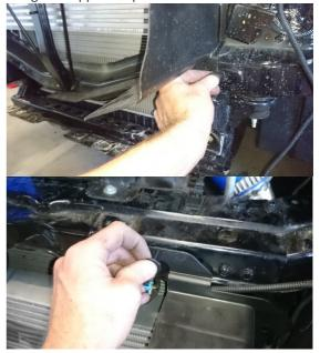
10. Reinstall the bumper reinforcement panel, lock panel supports and the lock panel.
