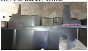
Reinstall air ducting by clipping into place using the supplied clips GM94215211.
