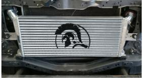
4. Reinstall the bonnet latch and brace. (NOTE – use the M6 x 10mm screw supplied in the kit to in the second hole of the brace as indicated in the image below to avoid core damage. As the brace is close to the core. There should be a gap of at least 5mm.)
