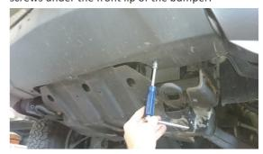
After all screws are undone carefully pry the bumper using trim removal tool. It is recommended to have a second person to help hold the bar to prevent damaging the bar during removal.
