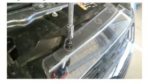
6. Next remove the screws under the wheel well connected the front bar.
