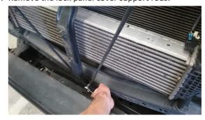
16. Remove the bonnet latch brace and unclip the sensor from the back side of the brace
