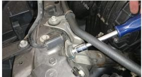
23. Undo and remove the hot pipe from the turbo.
