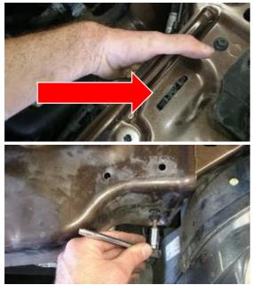
9. Reinstall air ducting by clipping into place and fasten using original bolt next to head light.
