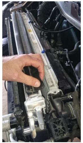
Reinstall the radiator core support panel and fasten using original bolts. Make sure the radiator lines up and slips in to the slot as indicated below.
