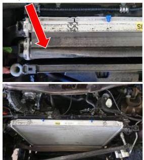
28. Remove plastic strip from the top of the OE intercooler and set aside to reinstall on the LEGENDEX intercooler.
