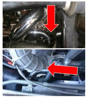
23. Next connect the silicone to the bottom of the turbo out let as shown in the image below.
