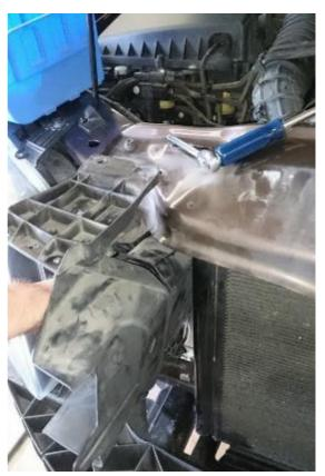
Carefully release the clips in the intake and remove forward from the vehicle and retain for reinstallation. Unbolt the radiator core support panel using a T-30 Torx screw driver (4 places on the front edge and 2 places on the top edge)
