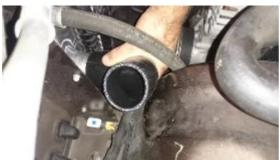
Next slide the silicone reducer (15A18923) on to the throttle body. Slide on clamps but do not tighten at this point.
