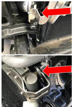
Install the M6x50 bolt and billet spacer
