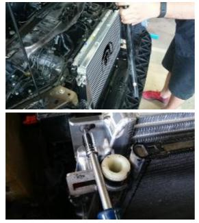
Reinstall the A/C condenser back in place being sure the lower tabs have connected properly and use the new M6 screws and washers to hold in place at the top. (only install 1 on passenger side at this time if your car has a the OEM transmission cooler)
