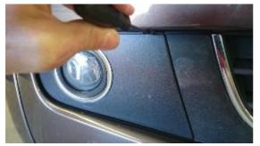
Remove the fog lamp retaining screws with a T25 Torx screwdriver. There are three screws on each side. Pull the fog lamps forward out of bumper and separate the electrical connectors. Retain for reinstallation.
