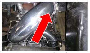
24. Ensure that the pipes do not rub anywhere and tighten up all clamps to tension.N.B. The OE plumbing may vary from auto to manual so please pay particular attention to ensure that there is no rubbing on other hoses. If you find hoses are touching insulate contact areas and zip tie to secure to ensure there is no rub through.
