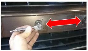
Remove the long bolts from fog light recess in the bumper using a 13mm Socket (1 each side). Retain for reinstallation.
