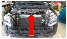
20. Remove the top intercooler hose buy undoing the clamps and force hose off. (If installing the LEGENDEX pipe kit it is suggested cut the hose along the length of the outlets using a knife to speed up the hose removal and Discard the OEM hoses).
