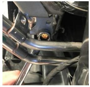
6. Secure the transmission cooler pipes to the bracket.
