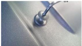
Remove the screws from under the wheel well using a T-25 Torx screwdriver (2 each side) and retain for reinstallation.
