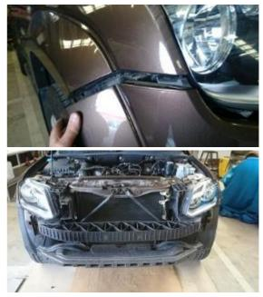
Undo and remove the radiator core support cross braces (2 places each) using a 13mm socket take care not to drop the spacer plate. Retain for reinstallation.
