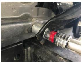
11. Reinstall radiator core support braces and the bonnet latch.
