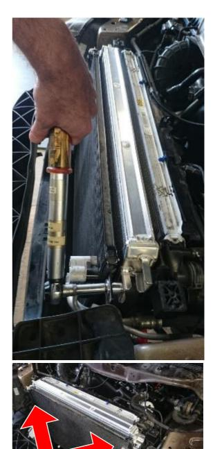
At this point reinstall the transmission cooler using the new screw supplied. This bolt is hidden as shown below. Ensure bottom mount is clipped in to the bracket.
