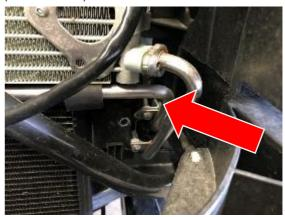
24. Undo mounting screw and release from lower clips and the clip behind as indicated below.
