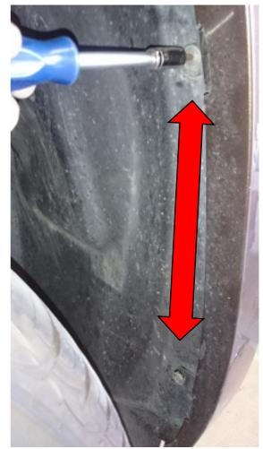
Remove the number plate and remove the two (2) bumper screws using a screw driver. Retain for reinstallation.
