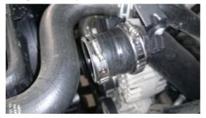
Next slip in tube 01.64398 and rotate into place to ensure silicone and hard pipes do not rub or touch anywhere. Then do up clamps to tension and confirm they are tight.
