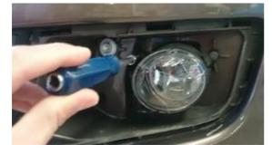
Remove the four (4) plastic scrivets at the top of the grille. Pry the center section of the scrivets upwards while rotating with Allen key and retain for reinstallation.
