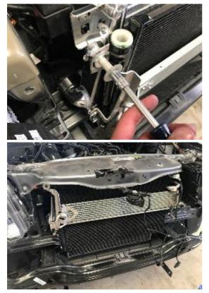
5. Reinstall the metal bracket to the LEGENDEX intercooler that hold the Transmission oil cooler pipes as shown.
