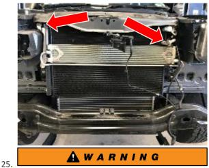
Take extra care during the next stage to avoid having to degas and re-gas the airconditioning system. Separate the Airconditioning condenser away from the radiator and intercooler assembly by pushing in the tabs on the top brackets and pulling up and forward out of the lower cradle. Do not remove but take up slack in A/C lines and pull forward. *Alternatively, have a qualified automotive air conditioning expert degas the A/C for removal.*
