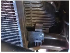
26. Once the A/C condenser is loosened undo the T-30 Torx screws on the Intercooler.
