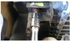
27. To remove lift up and forward. May require some manipulation of Radiator and A/C condenser and hoses to remove. It is suggested to have the help of a second person to spread the cores and hoses apart during removal to avoid damaging the radiator and A/C condenser cores by pulling in the direction of the red arrow as below.
