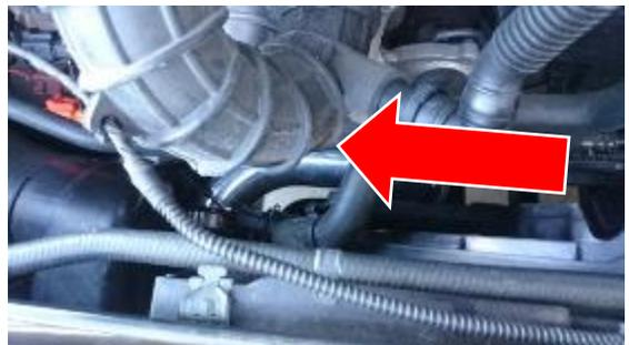
23. Next connect the silicone to the bottom of the turbo out let as shown in the image below.
