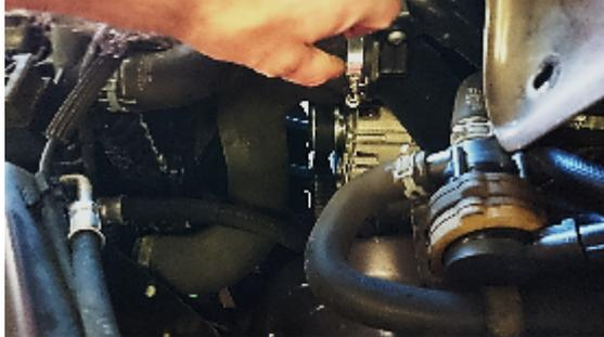
21. Undo and remove the bottom intercooler inlet hose by undoing hose clamps and either forcing the hose off (or if installing the LEGENDEX pipe kit cutting the hose away for ease of removal).
