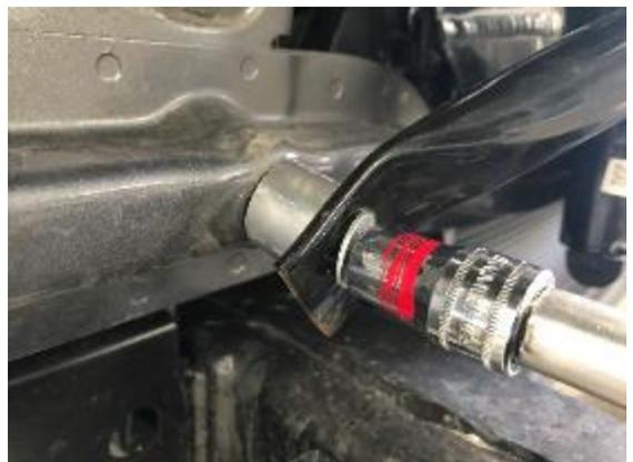
11. Reinstall radiator core support braces and the bonnet latch.
