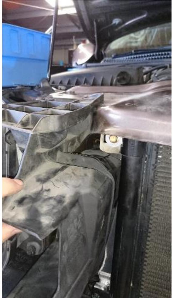
8. Reinstall the radiator core support panel and fasten using original bolts. Make sure the radiator lines up and slips in to the slot as indicated below.
