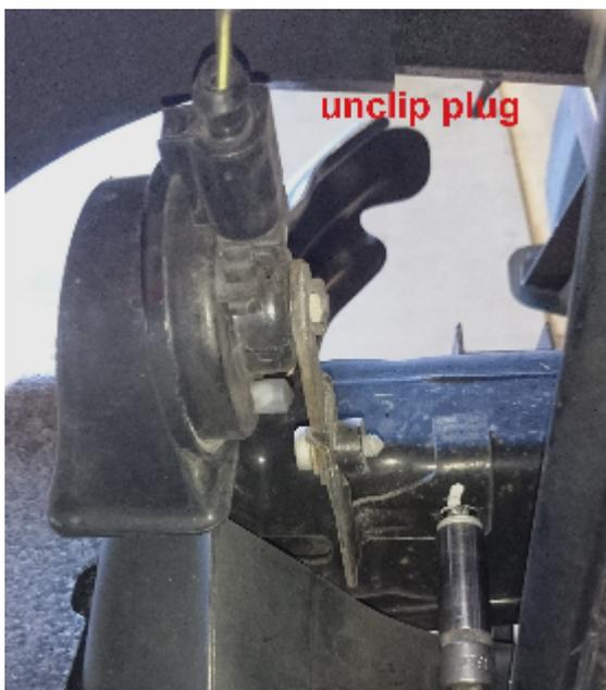
23. If your Amarok has the Automatic transmission cooler installed as shown below, undo the 2 mount screws holding the lines in place. If no transmission cooler is fitted proceed to step 25.
