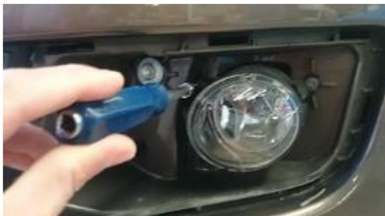
6. Remove the four (4) plastic scrivets at the top of the grille. Pry the center section of the scrivets upwards while rotating with Allen key and retain for reinstallation.
