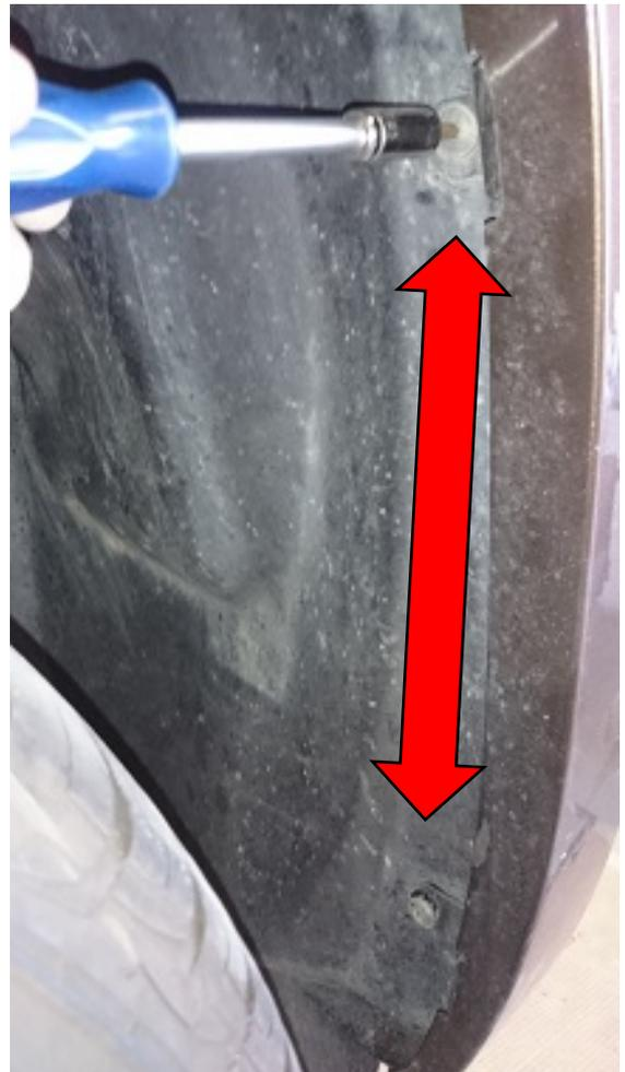
8. Remove the number plate and remove the two (2) bumper screws using a screw driver. Retain for reinstallation.
