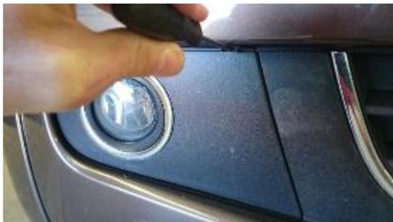
5. Remove the fog lamp retaining screws with a T25 Torx screwdriver. There are three screws on each side. Pull the fog lamps forward out of bumper and separate the electrical connectors. Retain for reinstallation.
