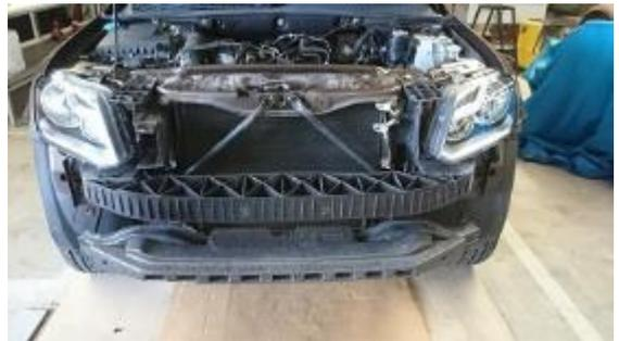
13. Undo and remove the radiator core support cross braces (2 places each) using a 13mm socket take care not to drop the spacer plate. Retain for reinstallation.
