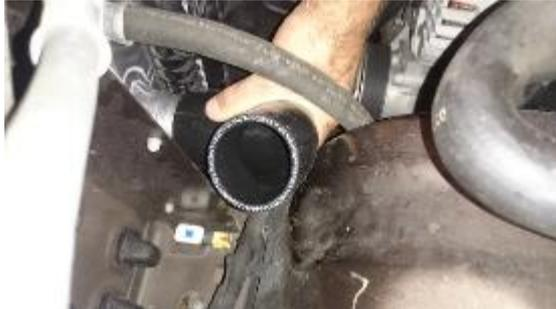
18. Next slide the silicone reducer (15A18923) on to the throttle body. Slide on clamps but do not tighten at this point.
