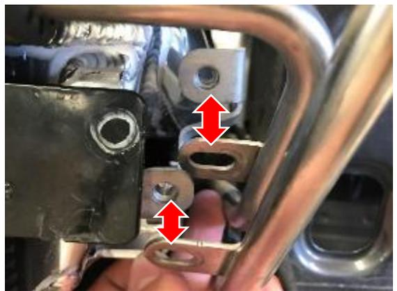
7. Reinstall the plastic strip on top of the new LEGENDEX intercooler.
