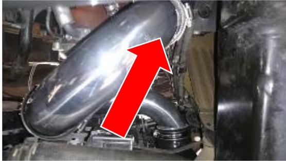
24. Ensure that the pipes do not rub anywhere and tighten up all clamps to tension.
