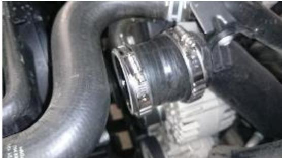
19. Next slip in tube 01.64398 and rotate into place to ensure silicone and hard pipes do not rub or touch anywhere. Then do up clamps to tension and confirm they are tight.
