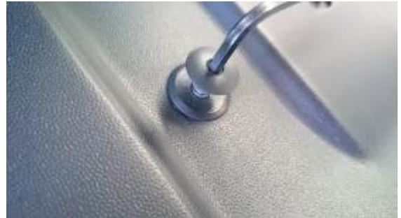
7. Remove the screws from under the wheel well using a T-25 Torx screwdriver (2 each side) and retain for reinstallation.
