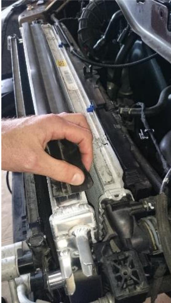
9. Reinstall air ducting by clipping into place and fasten using original bolt next to head light.
