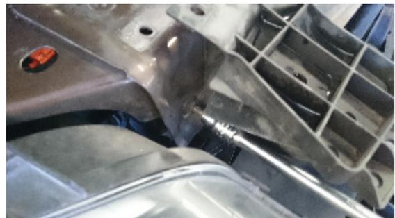
18. **NOTE** – Leave bonnet release cable connected to radiator core support and rest core support across the top of the engine being careful not to touch the battery or surfaces that may be easily scratched.
