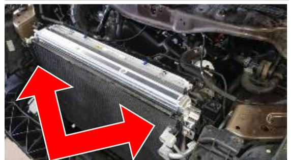
3. At this point reinstall the transmission cooler using the new screw supplied. This bolt is hidden as shown below. Ensure bottom mount is clipped in to the bracket.
