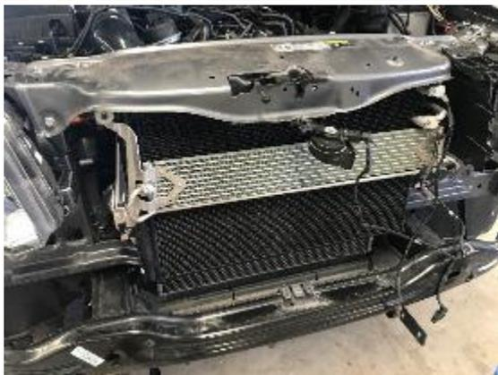
5. Reinstall the metal bracket to the LEGENDEX intercooler that hold the Transmission oil cooler pipes as shown.
