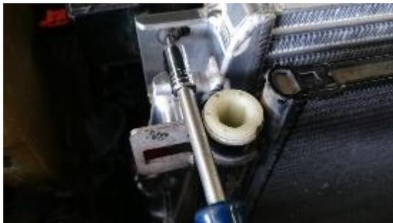
2. Reinstall the A/C condenser back in place being sure the lower tabs have connected properly and use the new M6 screws and washers to hold in place at the top. (only install 1 on passenger side at this time if your car has a the OEM transmission cooler)
