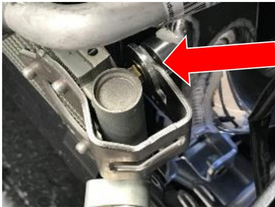
4. Install the M6x50 bolt and billet spacer 99A19837 on the driver's side to secure the AC condenser and the transmission cooler.
