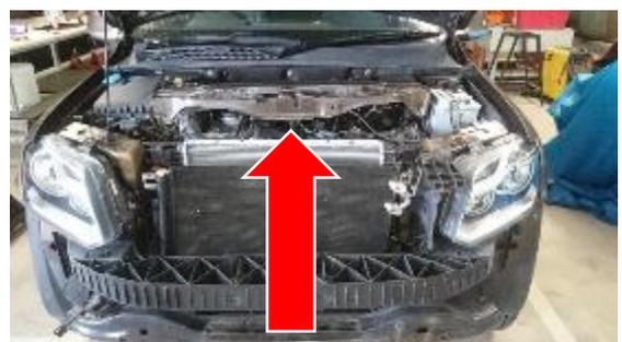
20. Remove the top intercooler hose by undoing the clamps and force hose off. (If installing the LEGENDEX pipe kit it is suggested cut the hose along the length of the outlets using a knife to speed up the hose removal and Discard the OEM hoses).
