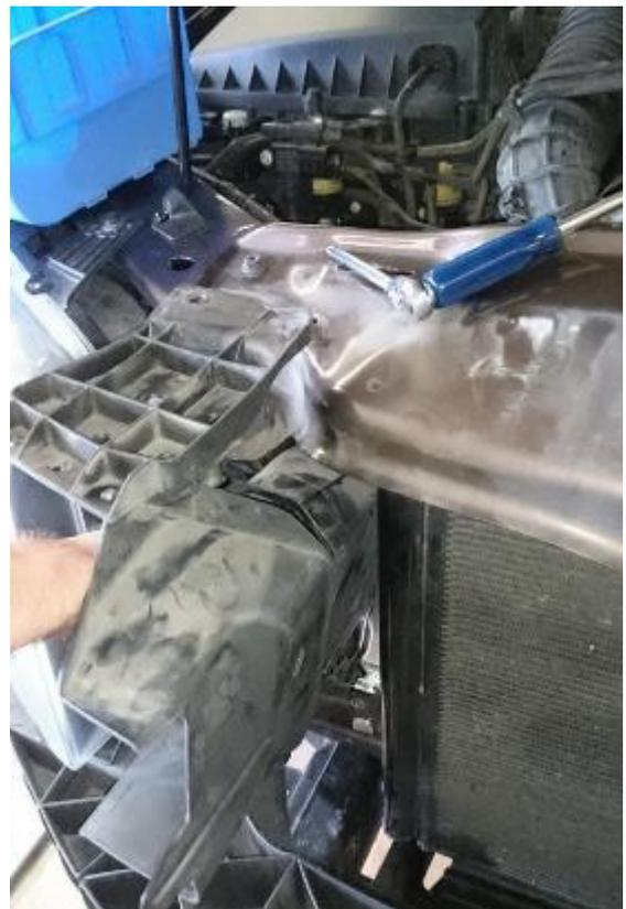
17. Carefully release the clips in the intake and remove forward from the vehicle and retain for reinstallation. Unbolt the radiator core support panel using a T-30 Torx screw driver (4 places on the front edge and 2 places on the top edge)
