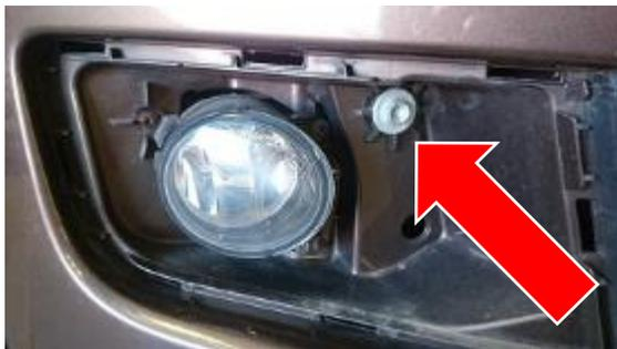
11. Remove the screws that retain the front edge of the wheel well liners to the underside of the bumper using a T-25 Torx screw driver.
