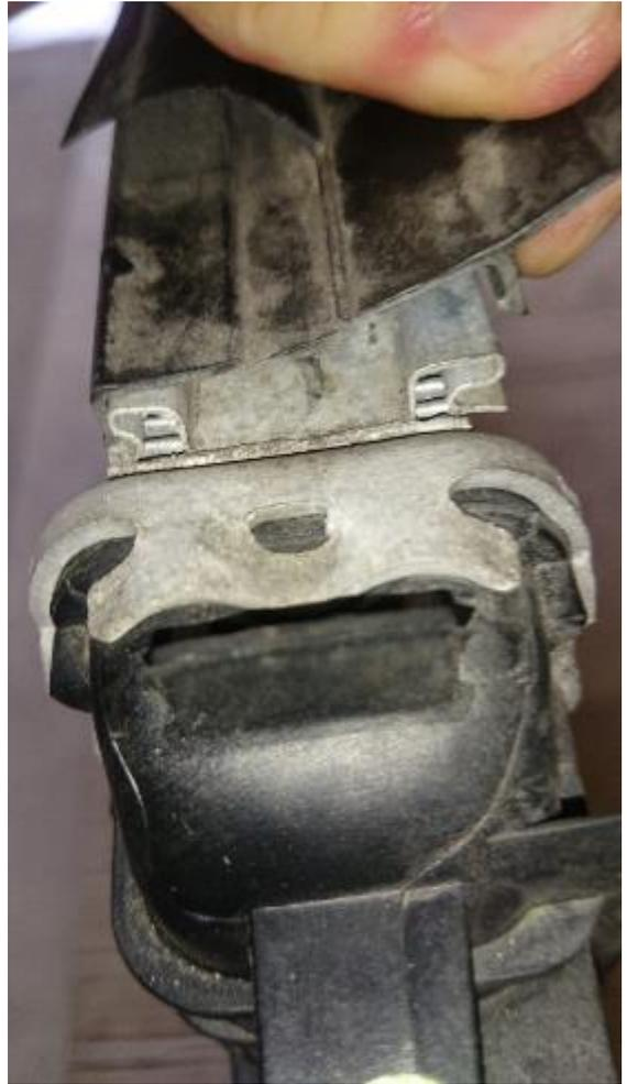
29. Also if fitted, remove the transmission cooler bracket as shown. Retain for reinstallation.
