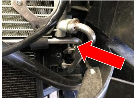
24. Undo mounting screw and release from lower clips and the clip behind as indicated below.
