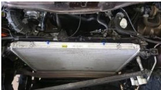
28. Remove plastic strip from the top of the OE intercooler and set aside to reinstall on the LEGENDEX intercooler.
