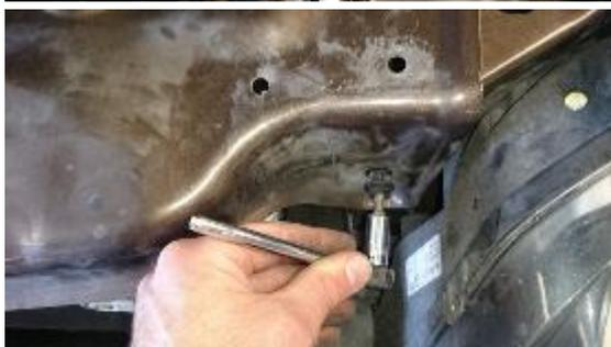
10. If you have the transmission cooler you may be required to install the supplied M8 x 40 bolts with the washers and 20mm spacers so the radiator core support braces do not touch the transmission cooler. In not fitted/required proceed to step 11.
