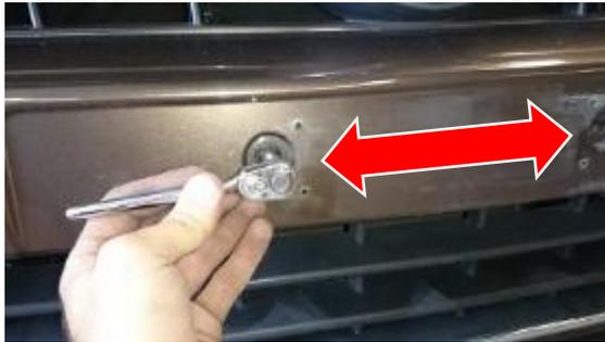
10. Remove the long bolts from fog light recess in the bumper using a 13mm Socket (1 each side). Retain for reinstallation.
