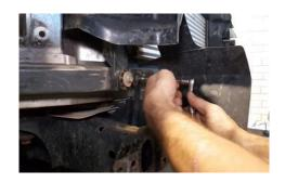
14. Tear away the plastic moulding that is between the chassis rail and the condensor.
