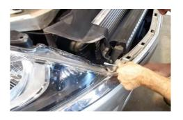
7. Undo the bolts holding the bottom of the bumper to the car.
