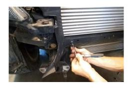
13. Remove the "L" shaped metal bracket mounted behind the air dam either side.
