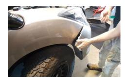
4. Remove the clips holding the top of the grill.
