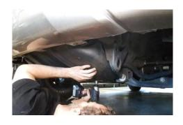
9. Carefully pull the bumper away from the car, taking care to disconnect the fog lights.
