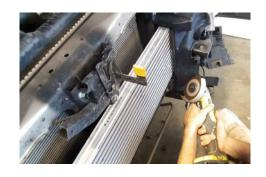
17. Remove and dispose of the bracket that secures the inner wheel liner to the body.
