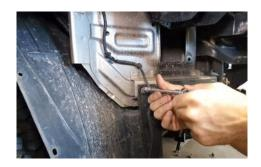
18. Trim the inner wheel liner as shown, following the angle of the metal.
