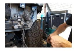
21. Now mount the bar bracket using the four factory bolts as well as eight of the supplied stainless nuts, washers and bolts.
