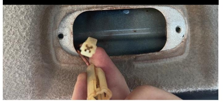
Next Up install the Light Bracket—Feed the two connectors into the Larger Centre Hole, one at a time.
