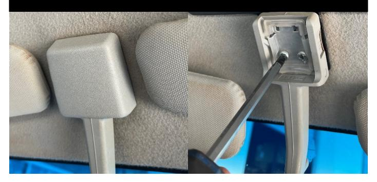
• Next remove the in-cab light. – KEEP THE SCREWS + all light components. – Disconnect the Battery to ensure you don't earth out. Or Use an Auto-electrician.
