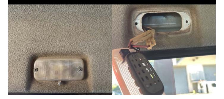
• Disconnect the Light from the harness, be careful not to lose harness behind cab.
