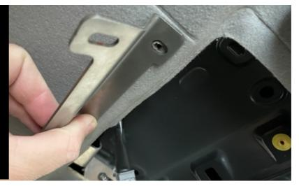
STEP 9 Loosely fit bracket with 6mm alan key bolt
