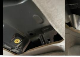
STEP 7 Loosely fit bracket with 6mm alan key bolt
