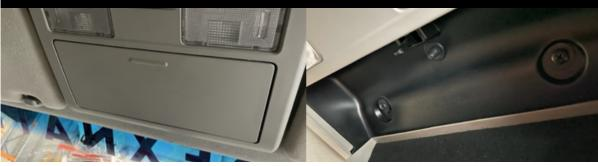
**STEP 3** Drop down plastic assemble and unplug wiring
