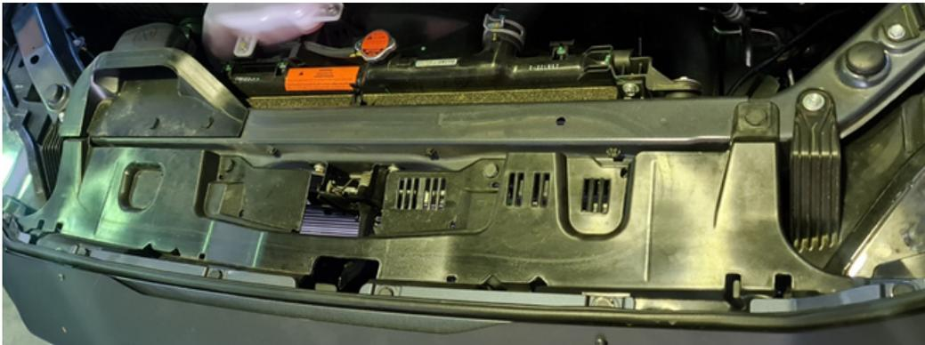
Various clips on the top of the engine bay area, Screw behind the logo, screws under the plastic flap shown in the image. Various bolts under the car. Remove the retainers holding the inner plastic arch to get access to inside and remove the bolts holding plastic bumper to car
