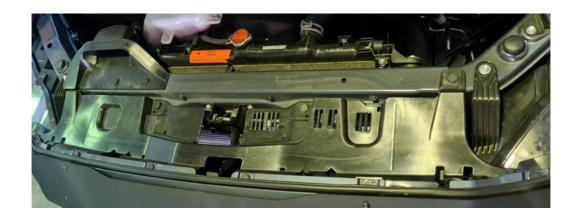
Various clips on the top of the engine bay area, Screw behind the logo, screws under the plastic flap shown in the image. Various bolts under the car. Remove the retainers holding the inner plastic arch to get access to inside and remove the bolts holding plastic bumper to car
