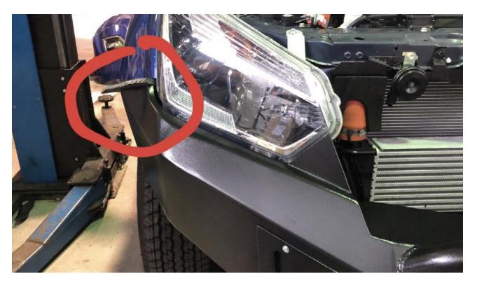
Typically, we cut the grille and apply some flat style pinch weld to get the bar nice and close to the car.
