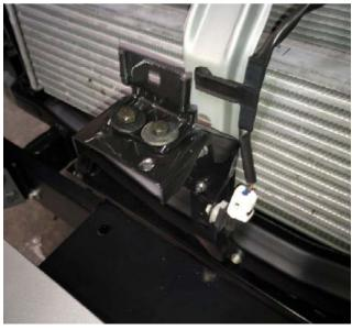
If you need further adjustment left to right you may need to flatten the bump on the chassis front member & install the Chassis collar bracket.
