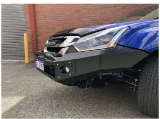
We recommend rubber pinch weld available on our store for \$29 or Clark Rubber to provide infill between bulbar and guards/headlights.
