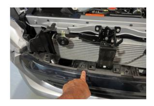
Remove the mud flaps from the left and right wheel wells. Then, remove the retention clips holding the inner wheel fender liners in place. Undo the nut attaching the inner liner to the mounting bracket and front bumper. The liner has been removed to show the nut location.
