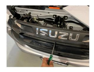
4 Remove the retention clips from the top of the bumper grill.
