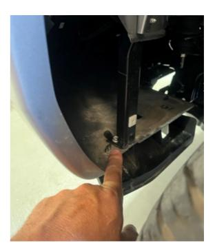
Remove the retention clip connecting the liner, bumper, and fender. The liner has been removed to show the location.
