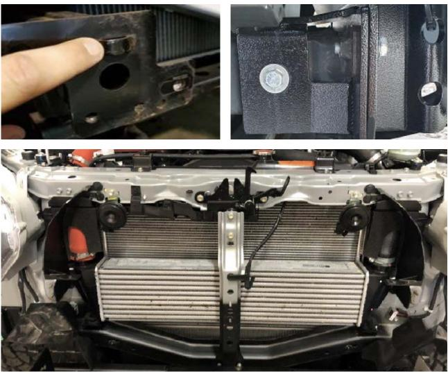
We recommend the use of 10mm foam on the sides between the bar and the car to help get the bar even.
