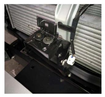
If you need further adjustment left to right you may need to flatten the bump on the chassis front member & install the Chassis collar bracket.
