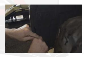
Pull away the wheel liner to unbolt the bumper from the front quarter panels.
