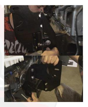
NOTE: When installing the chassis support bracket you may find your bar will move alignment. We suggest putting 10-15mm foam between bar and gaurds to keep bar inalignment.
