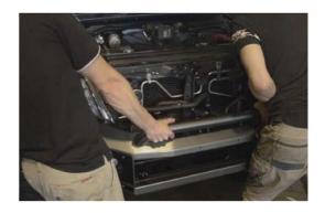
NOTE: Using 10-15mm foam will help you maitain even gap. You may wish to install rubber pinch weld bulb to fill the required gap for bar/cab movement. You should take care to avoid bar contact with headlight, you can check from under your 4wd to make sure sufficent space is kept. 10-15mm
