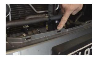
Unscrew the top of the bumper, Undo the bolts holding the lower part of the bumper as shown.
