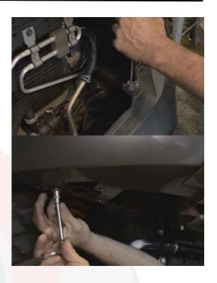
Remove the clips holding the inner wheel liner to the bumper
