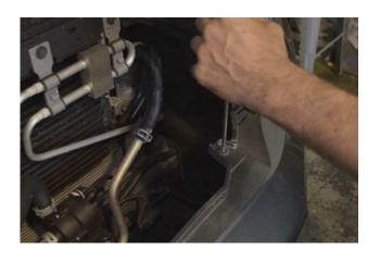
Undo the bolts holding the lower part of the bumper as shown
