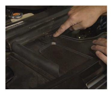
Pull the grill away, pushing the clips where it attaches to the bumper.
