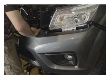
Remove the plastic white mouldings underneath the headlights. & side mouldings
