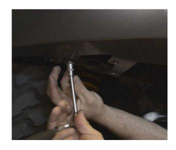
Remove the clips holding the inner wheel liner to the bumper
