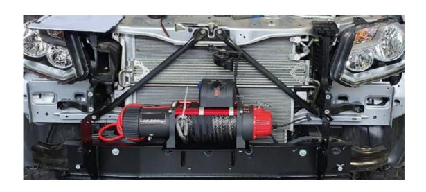
Once centered mark and drill out securing points under winch plate. Tighten lower bolts first in order to align cradle vertically.
