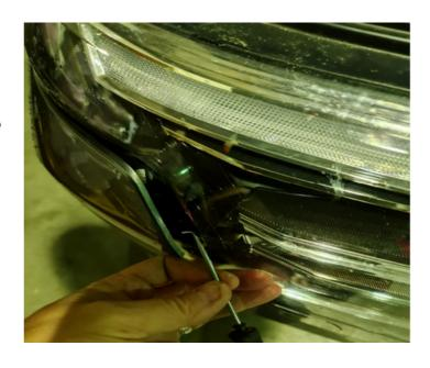
Remove the black bumper retainer shown in this photo held in by 2x 10mm bolt screws. Unclip all harnesses including the camera harness on the grille behind the badge. You will need to extend the harness for radar by unclipping the retaining plugs from the car.
