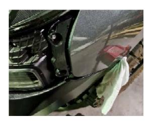
You will need take care with radar, avoid rattle gun vibration near it etc and try to keep unplugged for shortest time possible.
