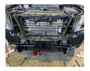
Remove the air dams near head lights or you can trim to suit profile of the bar which only possible by putting bar on marking and removing. If you are fitting a winch unbolt themiddle support bracket in the centre of the car above winch plate – Fits runva 11xp premium height.
