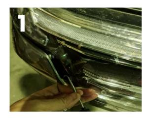
Remove the black bumper retainer shown in this photo held in by 2x 10mm bolt screws.
