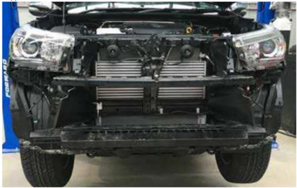
2) Install the cradle onto the chassis rail ends. Bolts should be finger Tight as you need to align the bulbar later.
