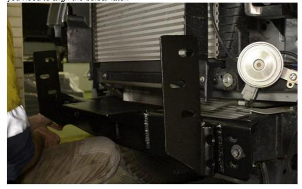
3) We recommend you bolt on cradle finger tight enough so you can move the cradle left to right if you need too. Use 10-15mm foam (clark rubber) or cardboard of equal depth and tape to the bulbar where bar meets guards, use a tape which does not affect the paint. See images below typical image
