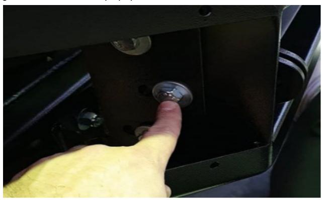
5. The black inner guards need to be trimmed to suit the profile of the bulbar and be secured in place so they do not move around.
