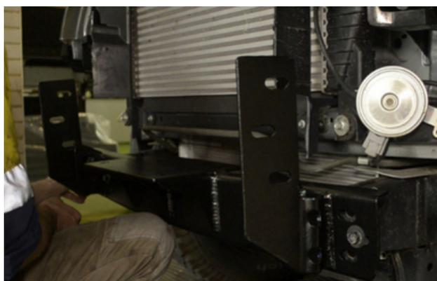
**INSTALL THE SUPPLIED CHASSIS REINFORCEMENT BRACKETS & COMBINED RECOVERY POINT**
