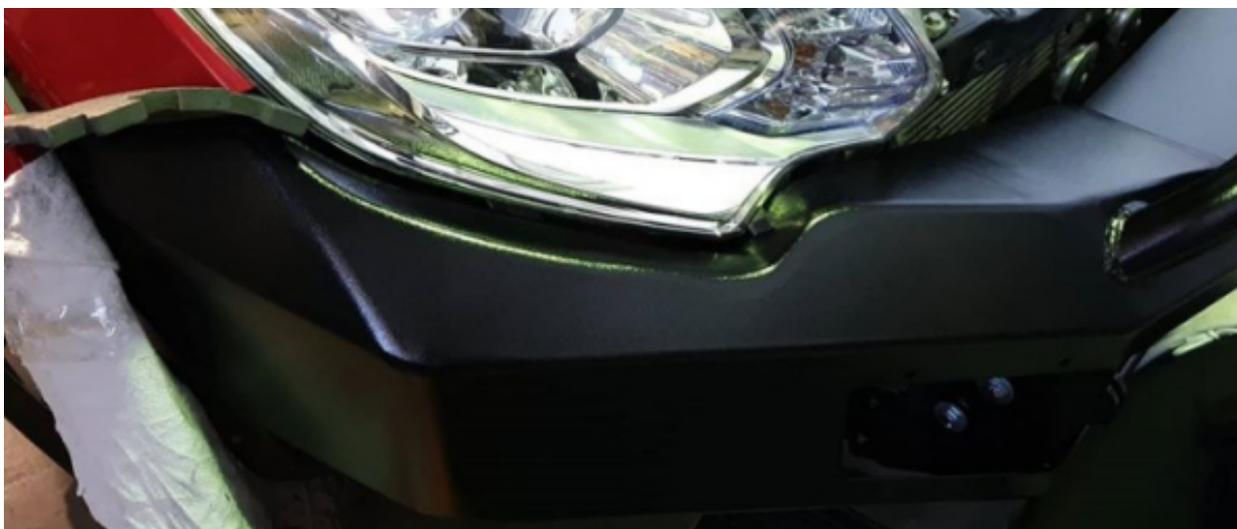
This will create an even gap on both sides, vs trying to align 1 side at a time. We also recommend using the same foam under the head lights to maintain the correct gap
