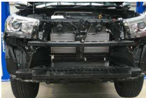
2. Install the cradle onto the chassis rail ends. Bolts should be finger Tight as you need to align the bullbar later.
