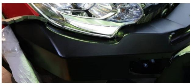
This will create an even gap on both sides, vs trying to align 1 side at a time. We also recommend using the same foam under the head lights to maintain the correct gap
