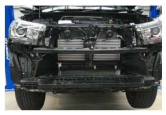
2. Install the cradle onto the chassis rail ends. Bolts should be finger Tight as you need to align the bullbar later.
