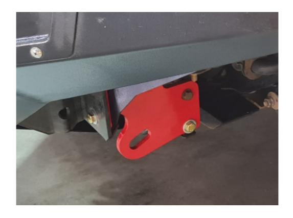
3. We recommend you bolt on cradle finger tight enough so you can move the cradle left to right if you need too. Use 10-15mm foam (clark rubber) or cardboard of equal depth and tape to the bulbar where the bar meets guards, use a tape which does not affect the paint. See images below typical image
