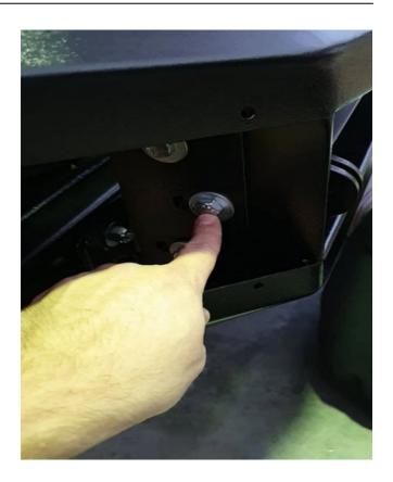
The black inner guards need to be trimmed to suit the profile of the bulbar and be secured in place, so they do not move around.
