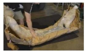
Remove the existing Bumper from the retaining clips located around the wheel arch and bonnet, in some models lower section may pot rivot on, remove and make sure neat with nothing protruding.
