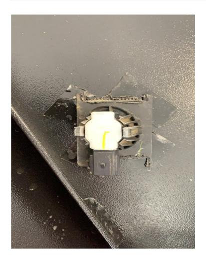
The sensors are removed from the old bumper and either double side tape to new bulbar or Sikaflex in place as below. Ensure you keep same locations and orientation
