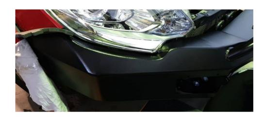
This will create an even gap on both sides, vs trying to align 1 side at a time. We also recommend using same foam under the head lights to maintain the correct gap You may wish to install Neoprene (CR) self adhesive tape 12mm Black or rubber bulb pinch weld on your bar to create flush sealed look. Rubber pinch weld available from clark rubber or our website.
