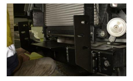
We recommend you bolt on cradle finger tight enough so you can move the cradle left to right if you need too. Use 10-15mm foam (clark rubber) or cardboard of equal depth and tape to the bulbar where bar meets guards, use a tape which does not affect the paint. See images below typical image
